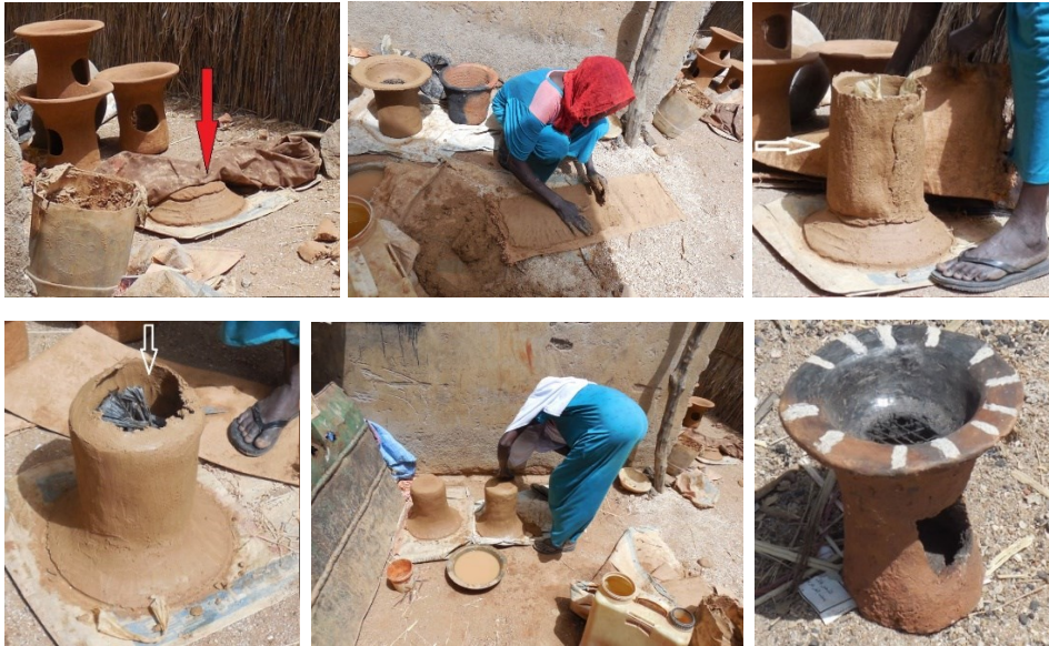
FIGURE 11: Forming a stove: rim; body; joining rim and body; forming the base; final shape of the stoves; decorated stove (photos by Hamdan 2020)
