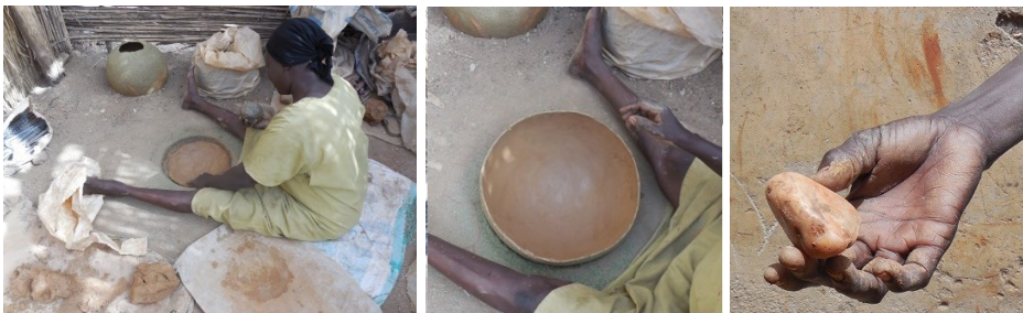
FIGURE 9: Forming the base of the water pot by making use of a negative mould dug into the ground; the base and a smoothing stone (photos by Hamdan 2020)
