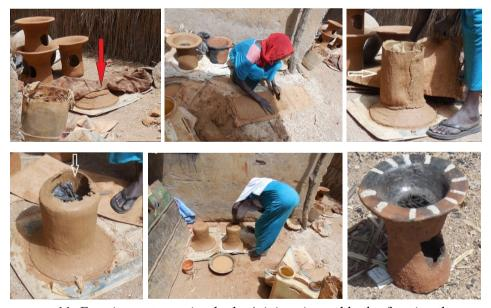
FIGURE 11: Forming a stove: rim; body; joining rim and body; forming the base; final shape of the stoves; decorated stove (photos by Hamdan 2020)
